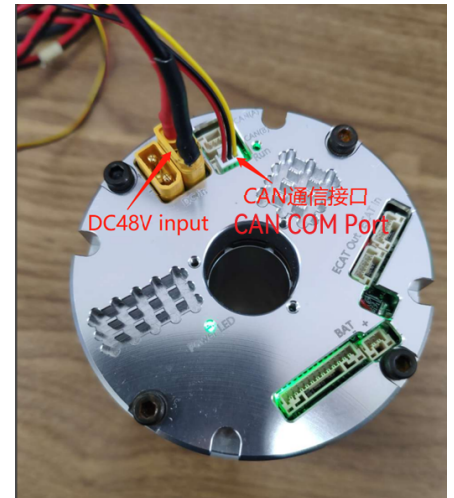
Figure 7-4 CAN wiring
